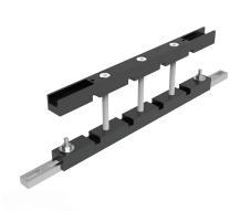
**Beskrivelse:** Busbar support up to 1600A to be mounted horizontally or vertically. Mounts directly to the enclosure frame or with help of CLPF profiles. Available in single and double bar per phase for bar thickness 5 mm and only single bar per phase for bar thickness 10 mm, and width from 25 to 80 mm.
